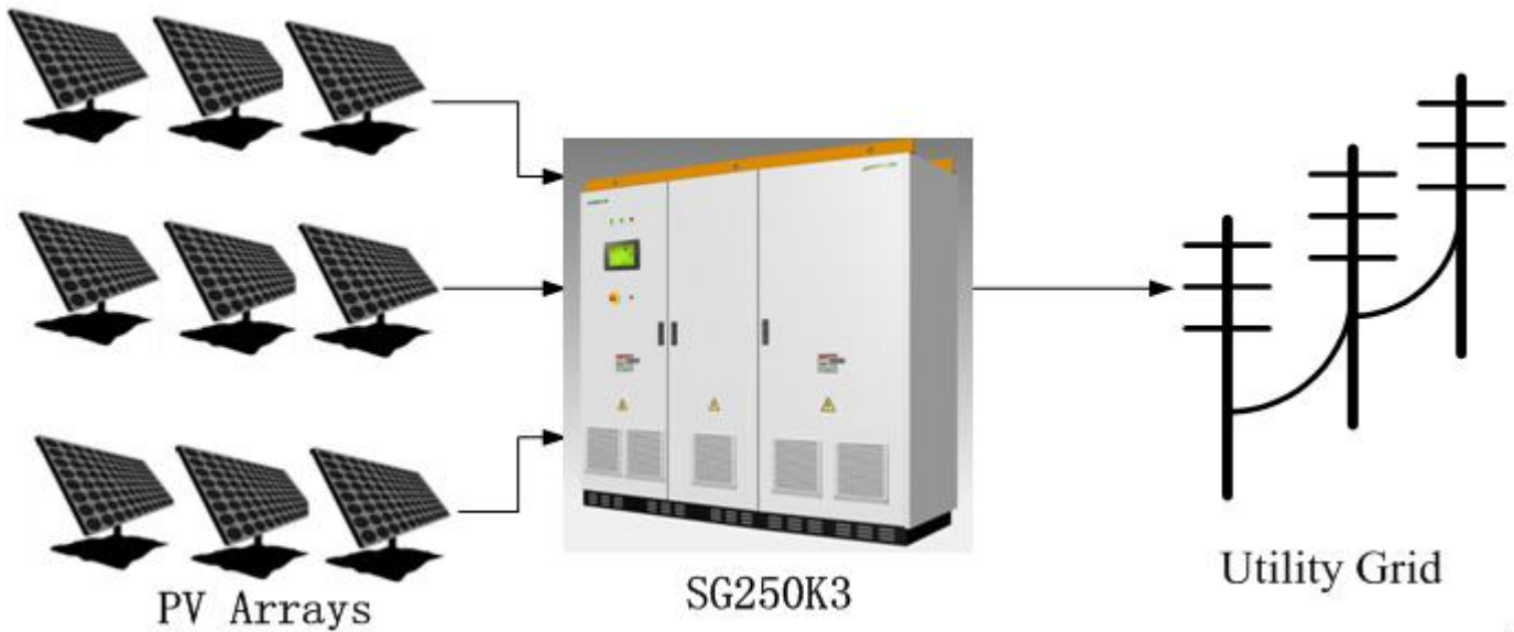
Figure 2-1 PV generation system with SG250K3
